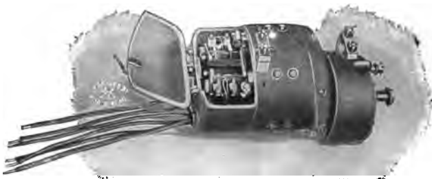
FIG. 291.—Type of General Electric Light Vehicle Motor, with case open, showing commutator and brush apparatus. The pinion end head is arranged for double reduction. Both end heads and gear housing are made of aluminum. Suspension by lugs to body. Capacity, 31\frac{1}{4} amperes at 39 volts; 1,800 r. p. m. at full load.
